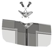
For the connection of the unit elements at the base frame, use the supplied M8 x 30 or M10 x 30 hex head screws. No brackets are used at these points.
